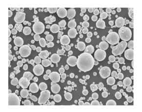
powder consolidation by hot isostatic pressing
