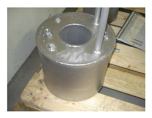
manufacturing of a HIP'd drum from a nickel alloy to save material and machining costs
