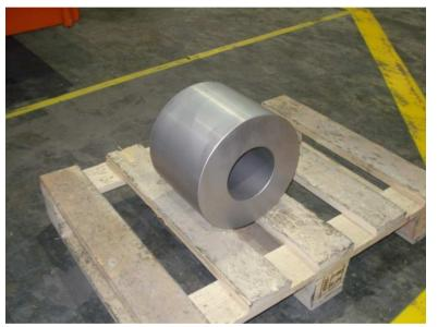
Canister material is perfectly bound to the base material by diffusion bonding. It can be removed by machining (simple shape) or by acid leaching (complex shape).
